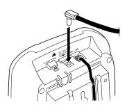
6. Route the adapter's cord through the narrow groove on the bottom of the bracket.
